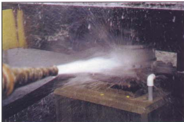
Hydrostatic load cells are washed down on a regular basis without fear of malfunction. They can be flooded or hosed down with no ill effects.
