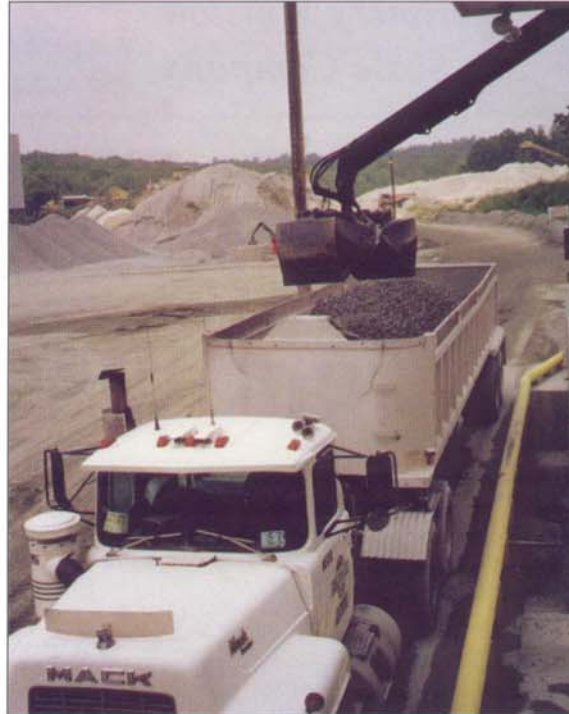
Top-off machine adjusts truck loads with trucks on the scale - one trip over the scale delivers exact weight.
