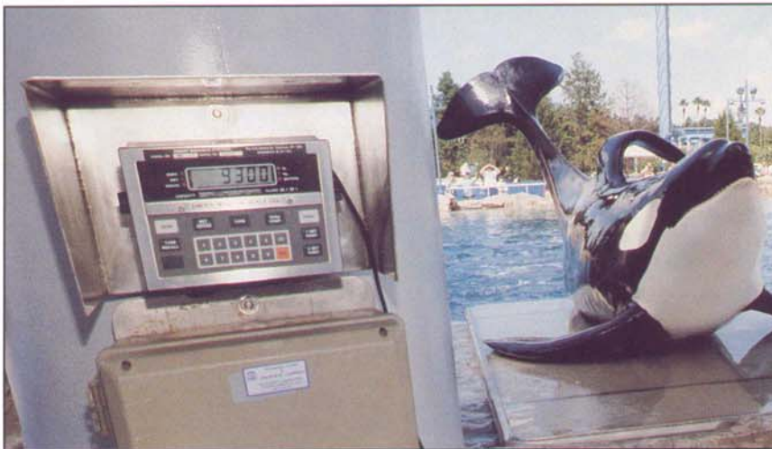
The digital indicator and the enclosed totalizer are housed outside, so the trainer can easily command the whale onto the scale while viewing the indicator.
