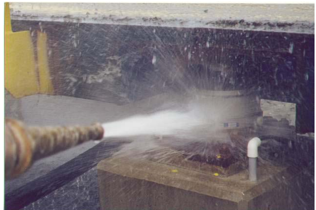
This load cell gets a direct blast from a high pressure hose.
