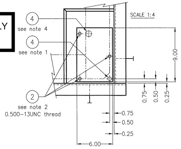
1" CONDUIT FOR (4) 1/8 OD HYDRAULIC TUBING, AND (1) 1/8 OD SHOP AIR TUBE. SUPPLIED BY OTHERS. USE EITHER LOCATION TO SUIT INSTALLATION.
